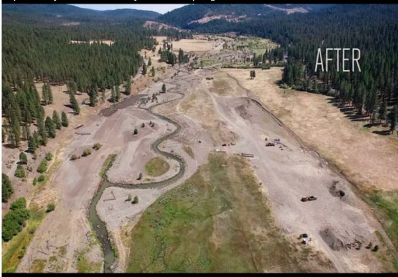
Before and after aerial images of channel realignment restoration actions implemented by the Confederated Tribes of the Warm Springs at the Oxbow Conservation Area.
